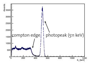
Due to energy conservation both photons have an energy which is equal to the electron rest mass (E = 511 keV). The photopeak represents the photons which deposited their entire energy in the scintillator (NaI) through the photoelectric effect. Less energetic events are the result of compton scattering.
