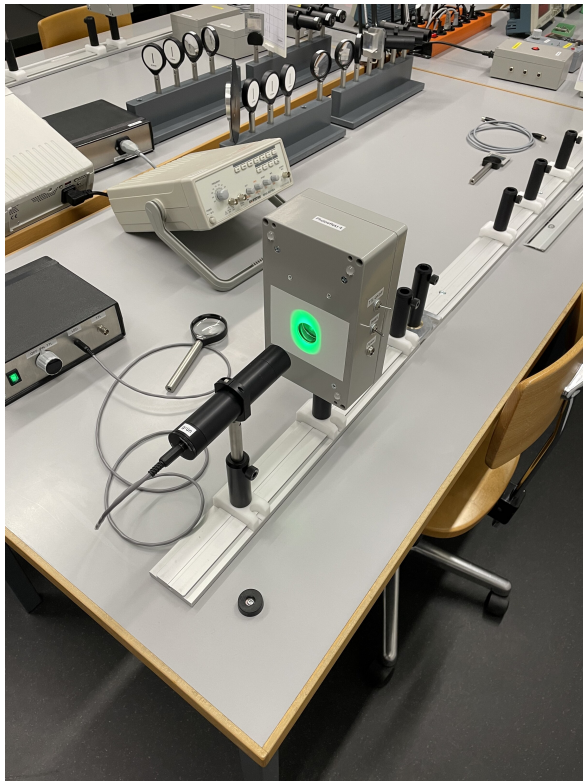
(a) Adjust the LED height to the photocell height.
