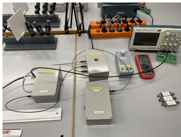
(b) Electronics overview: Power-supply, lock-in amplifier, normal amplifier, reverse voltage source, voltmeter, oscilloscope, low-pass filters.
