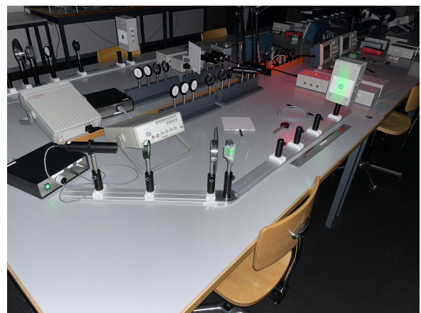
(d) Place the prism and align angle and height, s.t. light reaches photocell.
