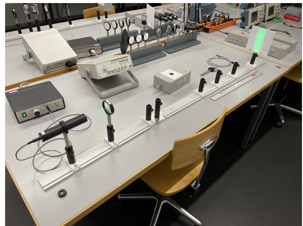
(b) Insert the first lens and collimate the LED in far field while keeping beam parallel to the table.
