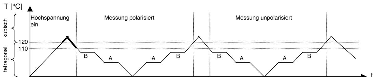
Figure 6: The horizontal parts A and B denote the measurements for the linear relation at constant temperature. Attention: When you turn off the oven the temperature is not constant immediately but can still go up or fall a few degrees.
