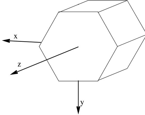
Figure 2: Orientation of the quartz unit cell in the coordinate system of the piezo module matrix. The x-axis coincides with one of the three polar twofold rotation axis and is called electric axis. The y-axis is called neutral axis.
