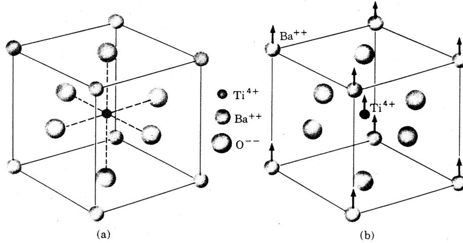
Figure 4: Structure of the cubic barium titanate and direction of the displacements of the lattice points to the tetragonal ferro electric phase.
