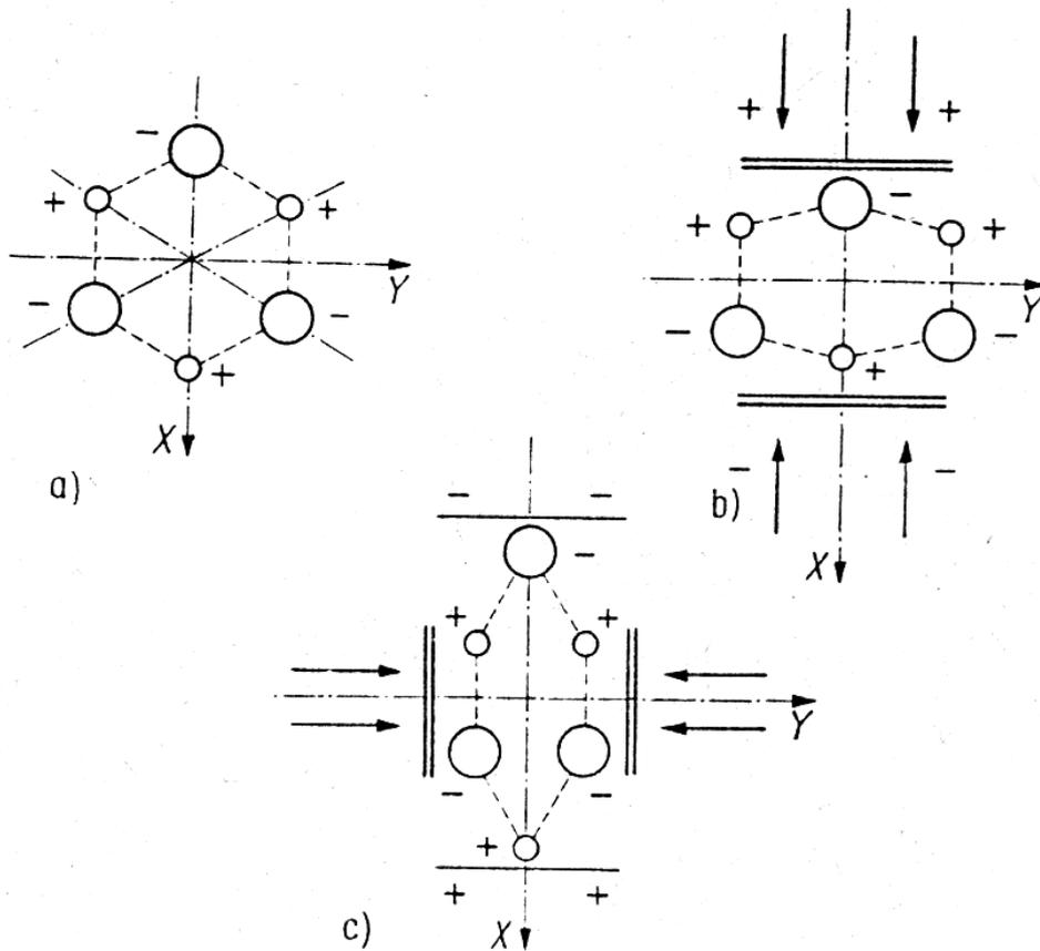
Figure 3: Structural model for the interpretation of the piezoelectric effect of quartz [10].
