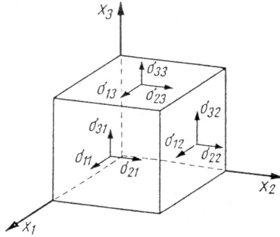
Figure 1: The components of the stress tensor [10].
