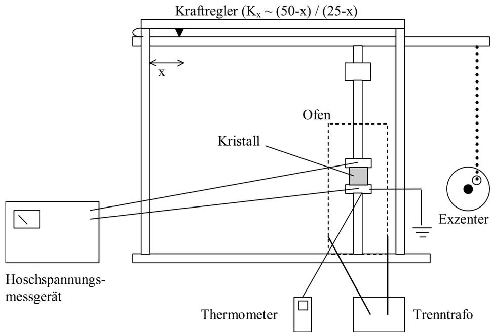
Figure 5: The measuring apparatus.
