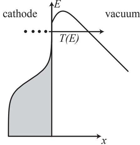
Figure 7: Schematic diagram of thermally activated tunneling from the heated cathode of the diode into the vacuum.
