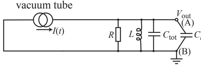
Figure 5: Measurement of the effective capacitance  $C_{\text{tot}}$
