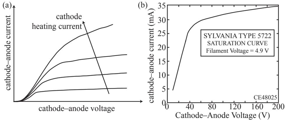
Figure 3: (a) Typical current–voltage characteristic of a vacuum diode for different heating currents. (b) Current–voltage characteristic of the vacuum diode used in this experiment (taken from the data sheet of the tube).
