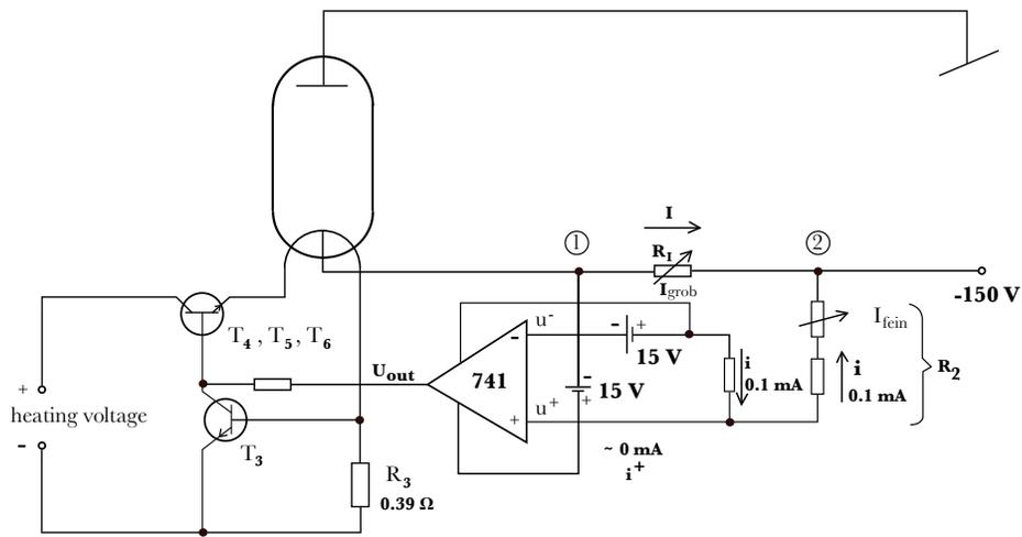
Figure 8: Scheme of the anode current stabilization circuit.
