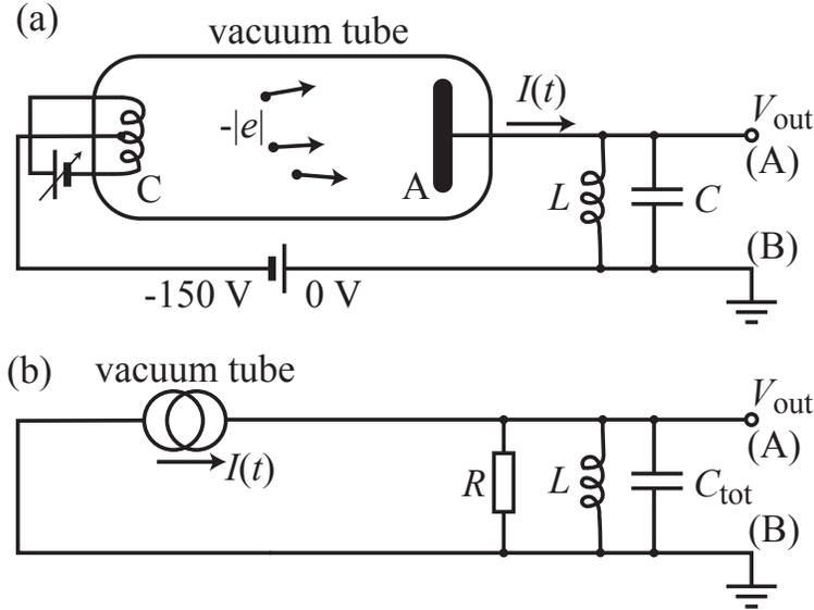
Figure 2: (a) Schematic circuit diagram of the noise generator. Within the vacuum diode, C denotes the cathode and A the anode. (b) Equivalent circuit of the noise generator.
