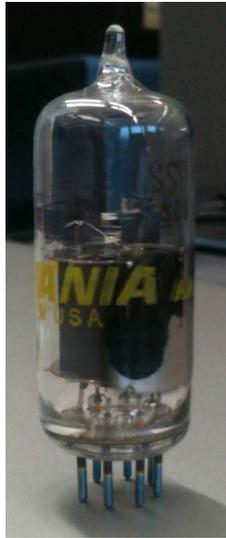
Figure 1: The vacuum tube used in this experiment for generating noise.
