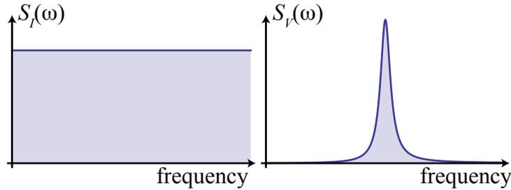
Figure 4: Left: White noise power spectral density of the shot-noise current. Right: Voltage noise power at the output (A) of the resonant circuit. The shaded area below this curve corresponds to the measured mean squared voltage noise.
