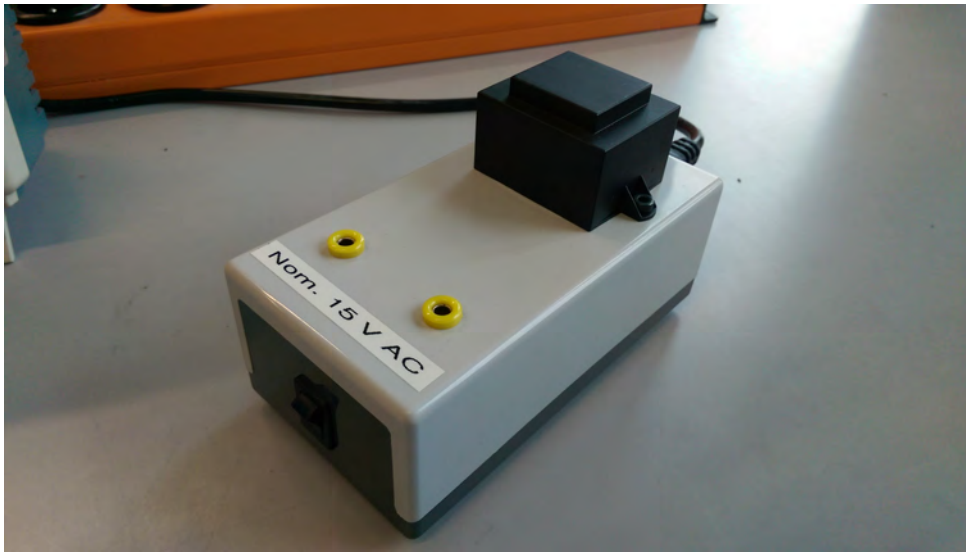
Figure 1.1: The 260V/15V transformer used in the experiment.
