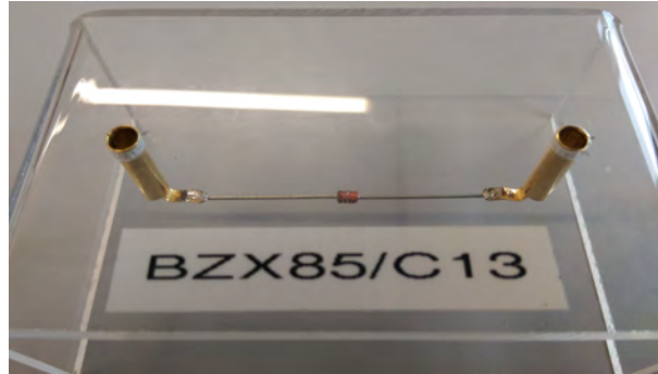
Figure 1.8: A Zener diode. The breakdown voltage is indicated as the last two digits of the part number.
