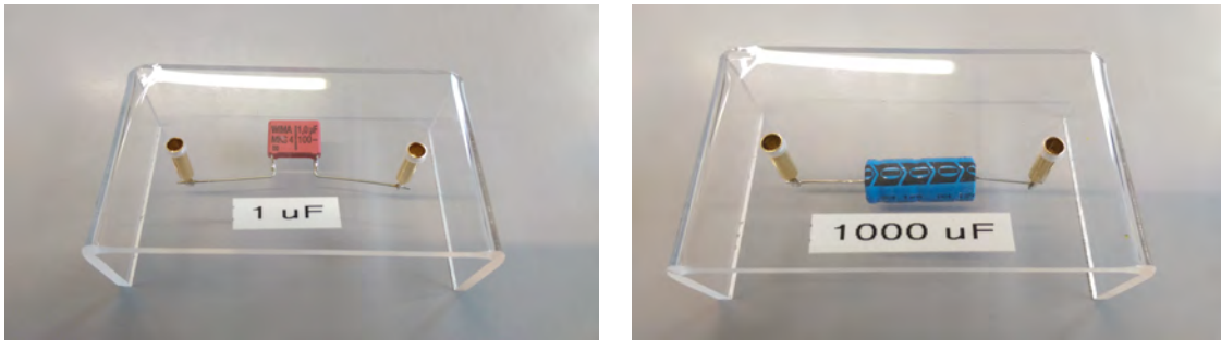
Figure 1.3: Two kinds of capacitors. Left: non-polarised ceramic; Right: polarised electrolyte.
